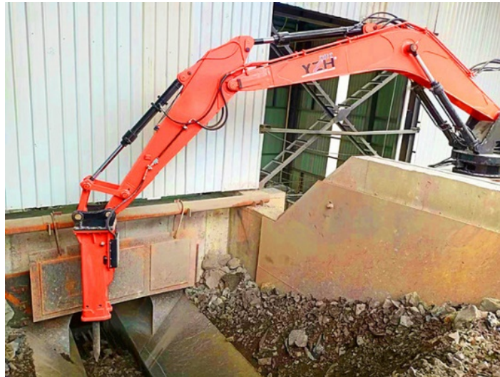
Figure 9. Hydraulic rock breaker
