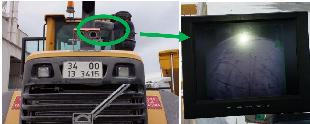
Figure 10. Proximity detection camera & monitor
